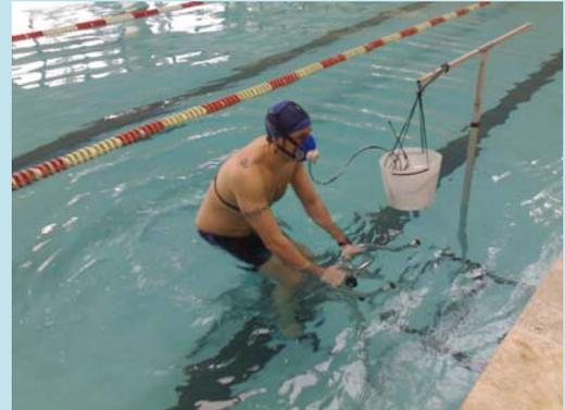
The resistance of the WSB, was set to obtain the maximum drag. The  $VO_2$  ( $ml \cdot kg^{-1} \cdot min^{-1}$ ) and the HR (bpm) were respectively measured by a portable K4b<sup>2</sup> gas analyzer (Cosmed srl, Rome, Italy) and Vantage NV heart rate monitor (Polar Electro Oy, Kempele, Finland).
